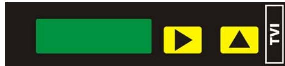
Push the buttons "►" + "▲": the display shows "Pro". Release both buttons, the display shows "P00" (which represents the number of the parameter) alternating with 4 digits representing its value.
